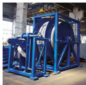
Reel for water jetting - a vessel (HLJV) for the construction of wind farms and maintenance operations
